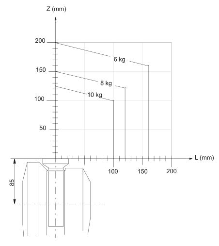
1.5.2 Maximum load and moment of inertia for full and limited axis 5 movement
